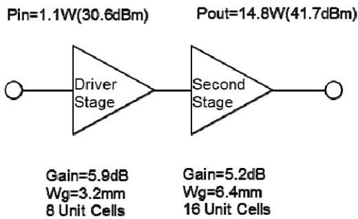
Fig.5 Block diagram of the 2-stage MMIC
