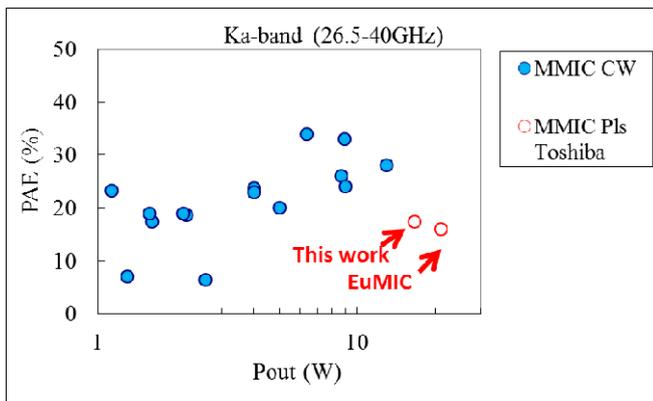
Fig. 8 PAE of GaN MMIC for Ka-band versus Pout.
