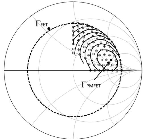
Fig. 3 Loadpull impedance of FET cell with pre-match circuit ( $\Gamma_{PMFET}$ ) and its de-embedded impedance ( $\Gamma_{FET}$ )
