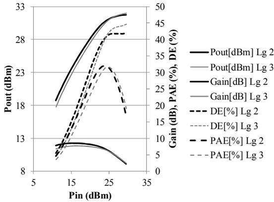
Fig. 4 Loadpull results of FET cell at 31GHz
