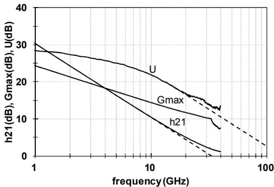
Fig. 2 h21, Gmax and Mason's U of the unit FET cells with 50 $\mu$ m-8-finger of Lg\_top=type2/Lg=type2
